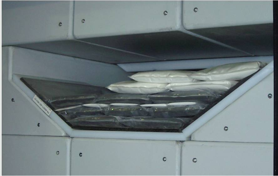
Non-symmetrical Loading is Duplicated in Factory Testing
